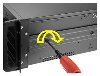
2. Unscrew all three screws on each side.
